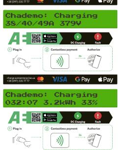
In car charging mode, the LCD display shows information about charging time, voltage level and current amperage.
