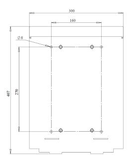
Figure 2. Mounting bracket
