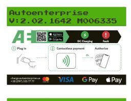
After the supply voltage is applied, the station display shows information about the software version and the serial number of the modem.
